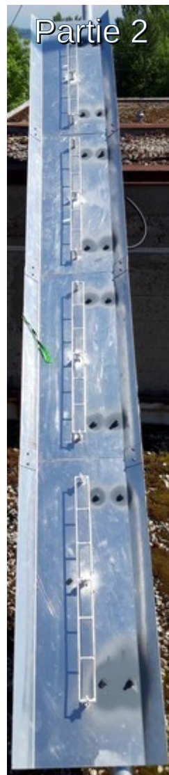
4x6 Quadlong 1296 MHz gain 20.2dBi Az.48° El.5.2°
