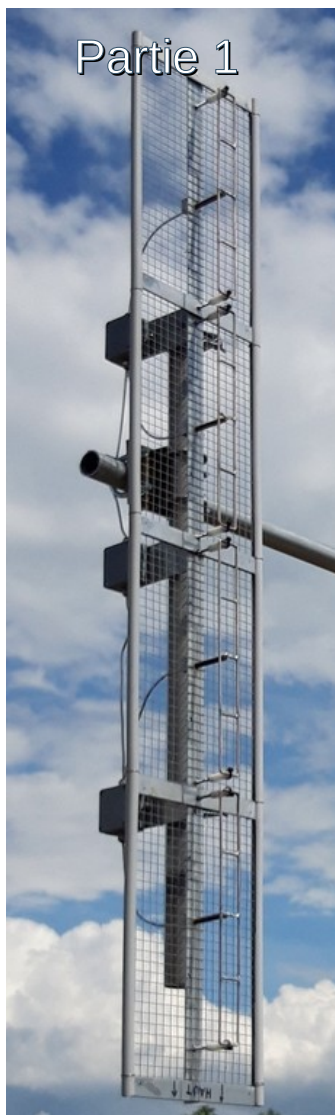
4x4 Quadlong 1296 MHz Gain 18.4dBi Az.61° El.7.4°
