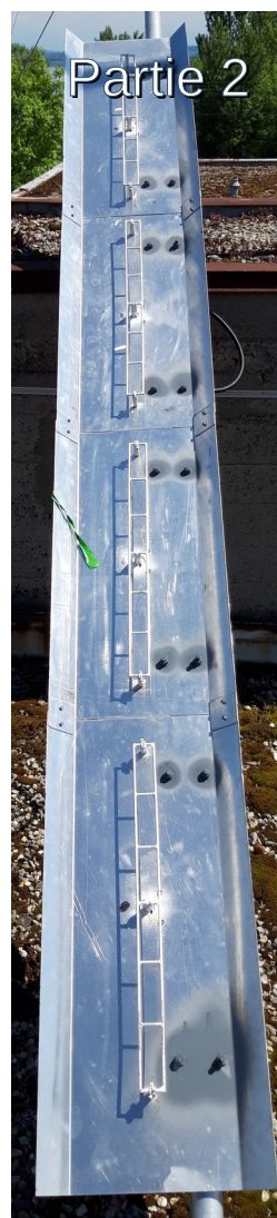
4x6 Quadlong 1296 MHz gain 20.2dBi Az.48° El.5.2°
