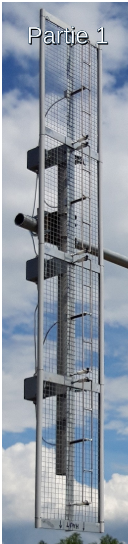
4x4 Quadlong 1296 MHz Gain 18.4dBi Az.61° El.7.4°
