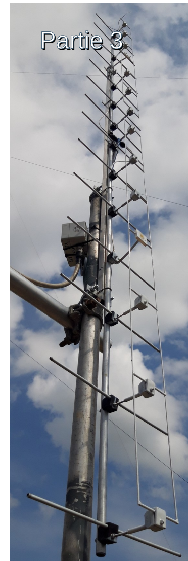
2x6 Quadlong 432 MHz gain 16dBi Az.71° El.11.4°
