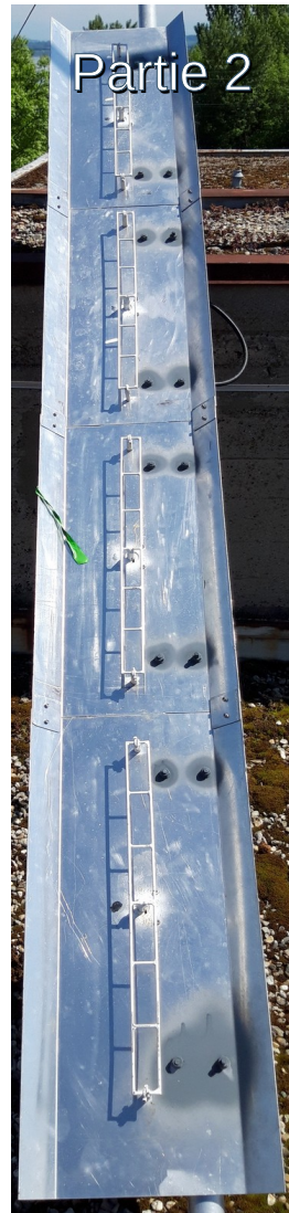
4x6 Quadlong 1296 MHz gain 20.2dBi Az.48° El.5.2°
